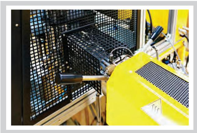
The heated connecting pipe from the extruder to the die and the access area into the blow moulding cabinet are covered with steel grilles to protect operators from accidental burning, Warning labels are attached to the steel grilles to alert workers of the danger of hot parts within the protective grilles. The enclosure will still allow the operator to see-through the grill sheet to check inside the moulding station.
