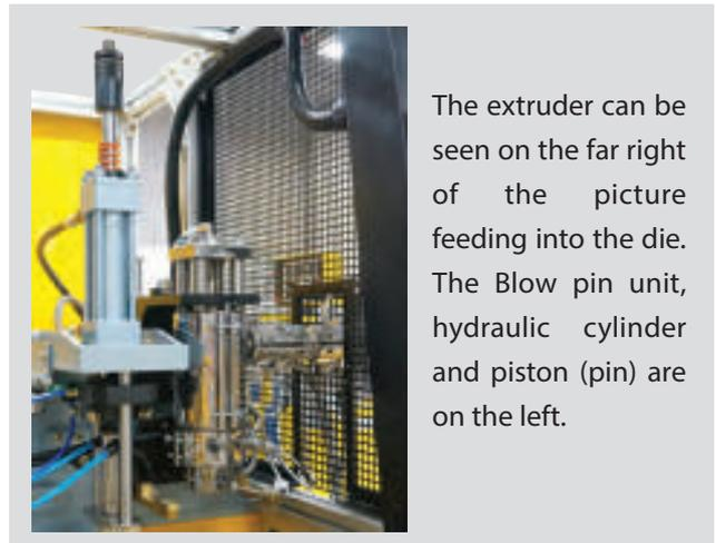
The extruder can be seen on the far right of the picture feeding into the die. The Blow pin unit, hydraulic cylinder and piston (pin) are on the left.
