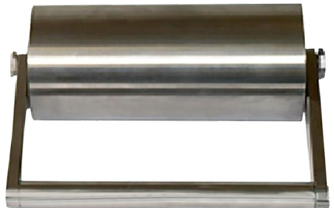
To determine the water absorption capacity of paper and corrugated cardboard (quick clamping grip)
