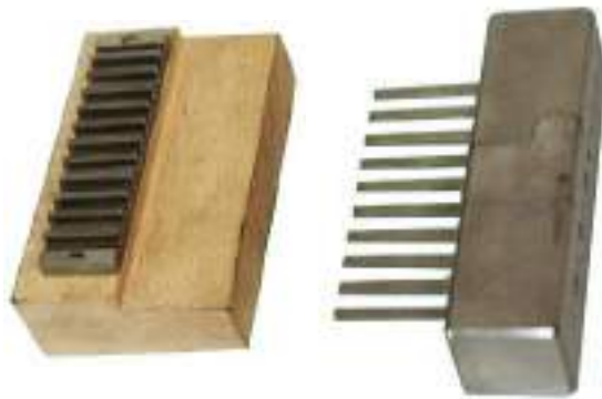
Device for gluing the ridges of corrugated paper samples to the adhesive tape
