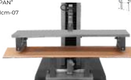
FLEXION TESTING FIXTURES (Corrugated Board) (3 and 4 Points of support) With fixed or variable support distances
