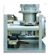
The optional variable speed drive for the strand feeding where control is done on a second digital instrument
