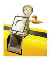
These extruders are also equipped with a built in high capacity vane-type vaccum pump. Including large inlet filters, as well as a vaccum dial gauge and release valve mounted on the top of the extruder barrel behind the vent opening.
