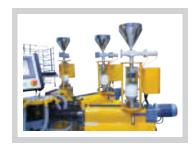
With our computerized weighing hopper feeder system it is possible to fully control the distribution of polymers in each layer of the film, both in respect to weight and thickness. The weighing hoppers will accurately control the amount of resin being fed to each layer using a closed loop system with the extruder speed control. And with the very easy-to- use central touch screen, the proportions fed from each extruder can be set individually or synchronously.
