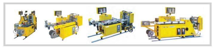
Our chill roll attachments are available in many sizes with roll widths ranging from 180 to 1200 mm and with either pneumatic or high-powered hydraulic lay-on of the top roll, and with many options.
