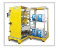
These stretching units are capable of producing film stretch ratios ranging from 3:1 to 10:1. Stretching of film is unidirectional - in the 'machine direction. The MDO unit is free-standing and can be used for stretching film supplied to it either 'in-line' from a working chill roll unit and extruders or "off-line" from a previously made roll of film.
