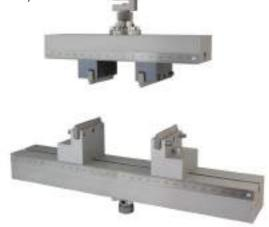
• **Fixture for Bending Tests at 4 Points** with spacing of adjustable lower supports up to 300 mm (according to GRCS specifications)
