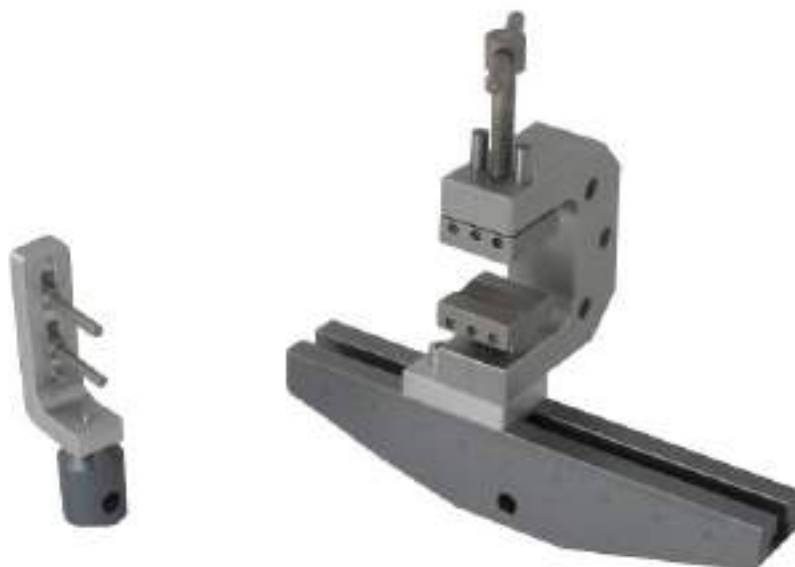
Special syringe holder for the 90° bend test
