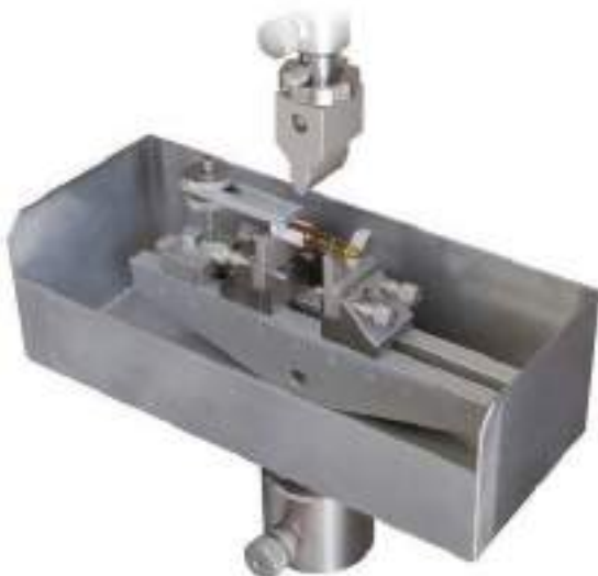
Test fixture with a tray for the collection of fluids from the blisters.
