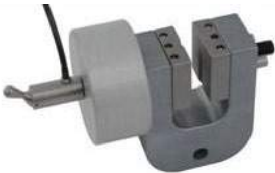
Pneumatic grips equipped with manual microswitch
