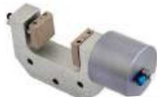
Pneumatic Grips model MDN-0,6/50- Ko (1 pneumatic piston)
