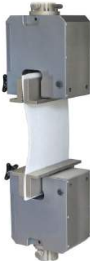
MDN/20+BW200: Wave Jaws 60 x 200 mm, testing a carpet / rug sample
