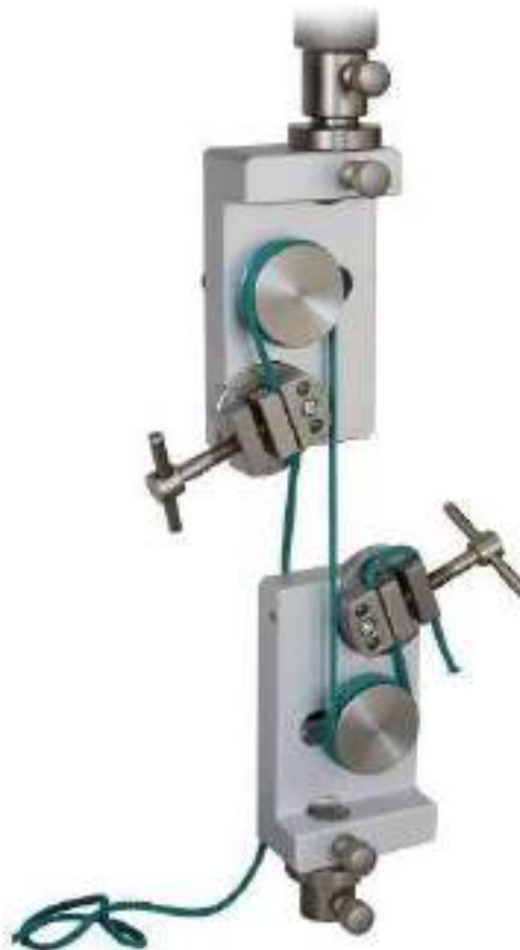
MB-N/5-VI+BD+D40 Jaw angle and distance from bollard to center line adjustable
