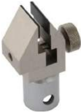
MTP/100-25-F-BG Jaw width 25 mm rubber coated
