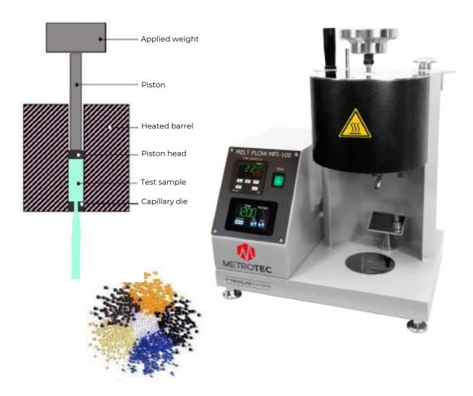
The fluidity index is a basic rheological test that is performed on a polymer to determine its fluidity. It is measured in g/10min. It is defined as the amount of material (measured in grams) that flows through the hole of a capillary die in 10 minutes, maintaining constant pressure and standard temperature.
