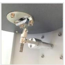
Set of 7 chrome and polished weights included in the standard supply: 1,2 Kg - 2,16 Kg - 3,8 Kg - 5 Kg - 5 Kg - 6,6 y 10 Kg
