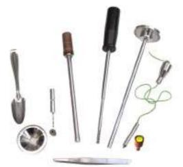
**Spatula** and pellet feeding **funnel**, Tungsten Carbide Ø 2,095 mm **capillary die**, Capillary die **cleaning tool**, **Piston**, Cylinder **cleaning tool**, **Extrusion tool**, **Plumb line**, **Bubble level** and **Tweezers**.
