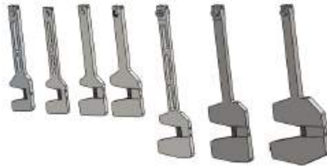
CHARPY Impact Hammers according to ISO standards
