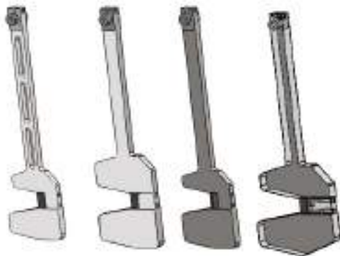
CHARPY Impact Hammers according to ASTM standards
