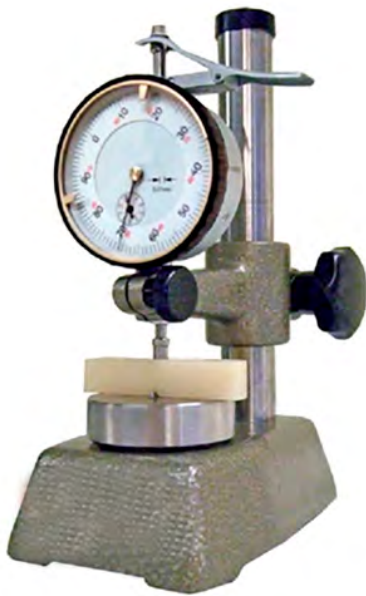
ANALOG MICROMETER MIP-20 (resolution 0.01mm) Verification of the depth of the “V” notches
