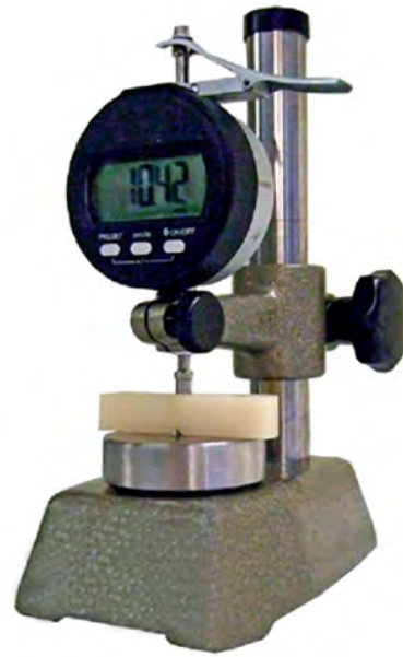
DIGITAL MICROMETER MIP-20D (resolution 0.01mm) Verification of the depth of the “V” notches
