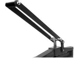
The Model MP-15 and MP-25 presses, due to their long cutting length of 300 mm, use a special double lever system, requiring very little effort to cut the samples.
