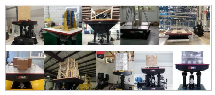
Hydraulic Vibration(HV) Systems perform the repetitive bounce, sine sweep, resonance search and dwell, and random vibration tests that help you:
