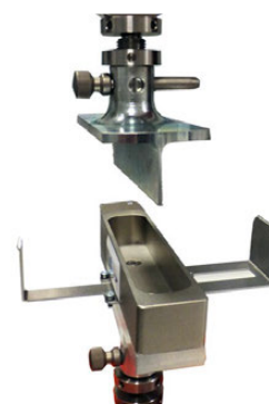
FLEXION TESTING FIXTURES (Corrugated Board) (3 and 4 Points of support) With fixed or variable support distances
