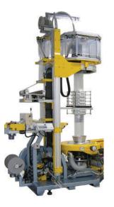
The film towers are made to suit the specific co-ex film blowing line in respect of die size, number of layers and extruders, as well as required output. The nip-roll width of the towers varies from 250 to 600 mm and all towers have motorized height adjustments. The maximum height is made in accordance to customer requirements, but as an example our largest 600 mm tower has a standard height range adjustable from 3.2 to 4.2 meters.
